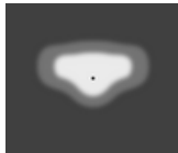
[T3] Type III, Asymmetric, Side throw - 143x68°
