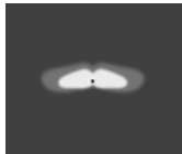
[SLS] Special linear, Side throw - 145x45°
